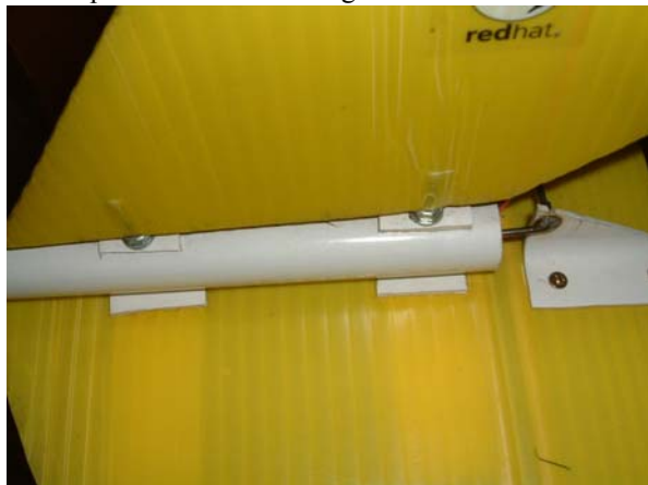
Switch mounting detail (vertical & shutter forward) to avoid accidental switch off.
