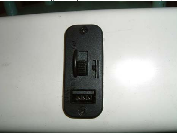
Switch mounting detail (vertical & shutter forward) to avoid accidental switch off.
