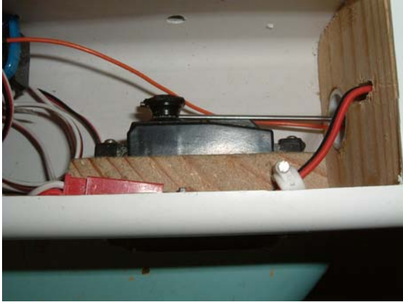
Throttle servo mounting detail
